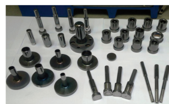
DLC coated tools for extrusion
